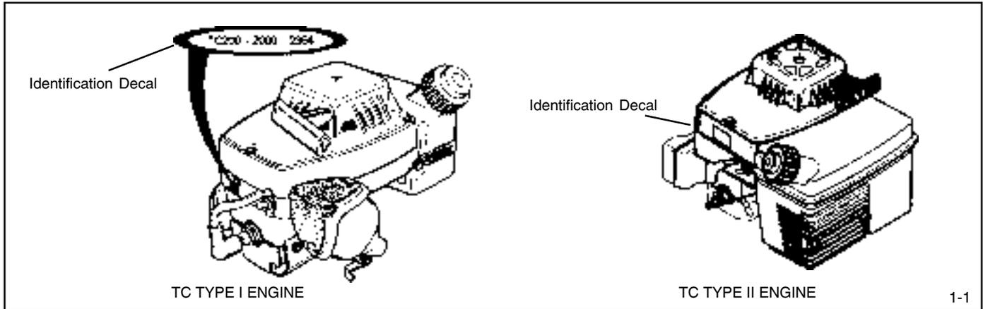
The engine identification decal will include the model number, specification number, warranty code, and date of manufacture (diag. 1-2).
