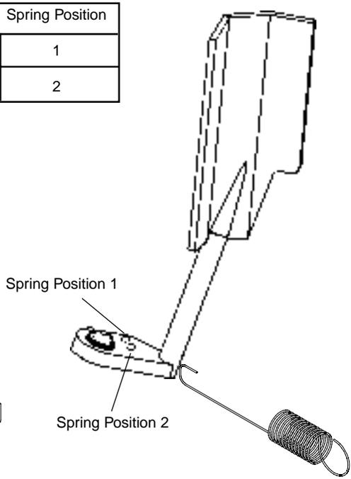
Adjust governed high speed with speed control plunger pulled back against speed adjustment screw
