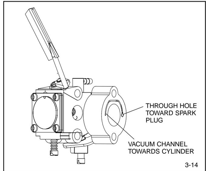
**NOTE:** Do not re-use old choke or throttle plate shutter screws. New screws are treated with a dry Loctite adhesive to secure them in place.
