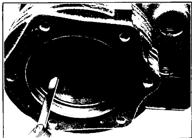
Figure 7-9. Checking Ring End Clearance in Bore
